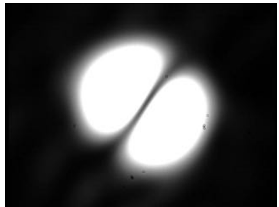
Modes: TEM_{01} Laguerre–Gaussian or TEM_{10} Hermite–Gaussian Skew: \frac{\pi}{4} rad or TEM_{01} Hermite–Gaussian Skew: -\frac{\pi}{4}
