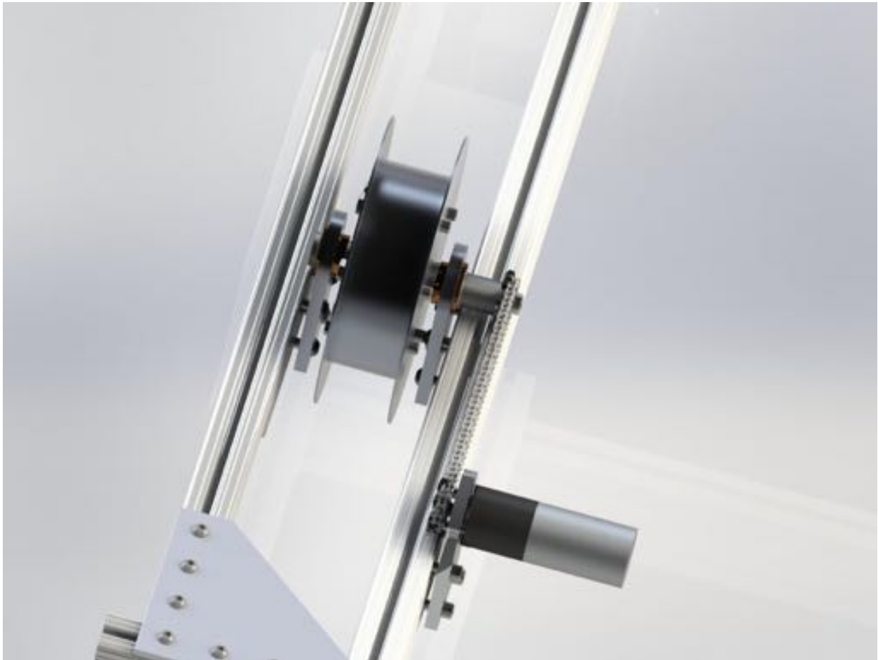
Figure 13: Solidworks render of DC motor chain drive
