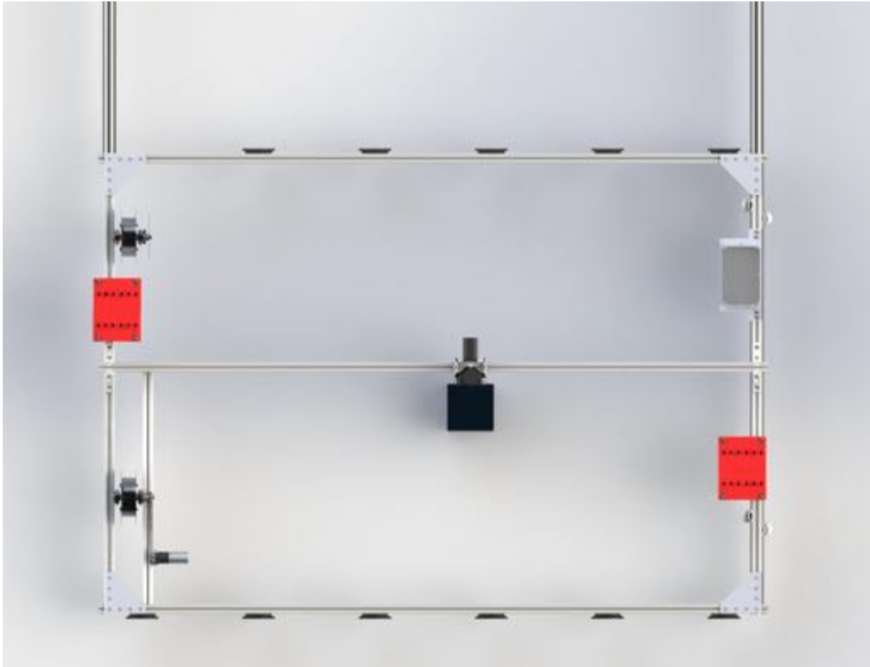
Figure 29: Top down view of chassis with chain drive
