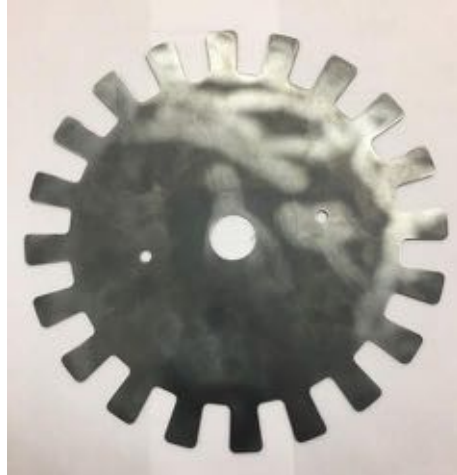
Figure 24: Encoding disk, proximity sensors outputs high when in front of tab and low otherwise
