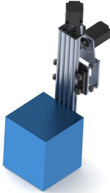
Figure 3: Mechanical configuration of stepper motors and mounted Crop Sense (blue box)
