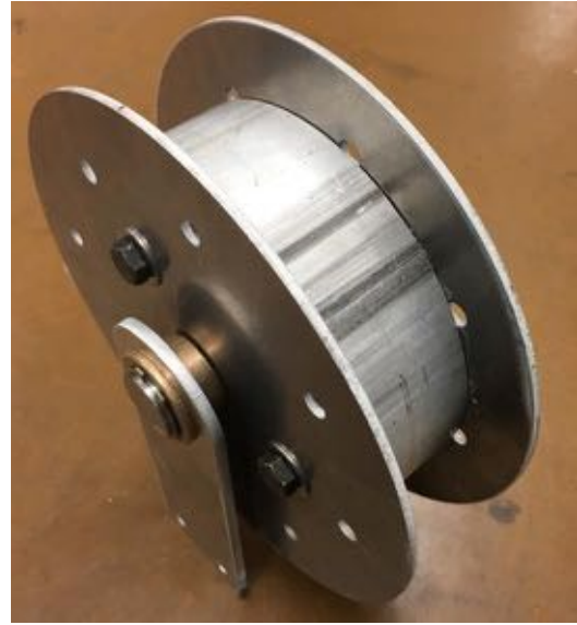
Figure 10: Completed flanged wheel
